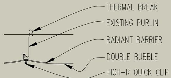
**HIGH-R® Radiant Double Bubble Solution**
