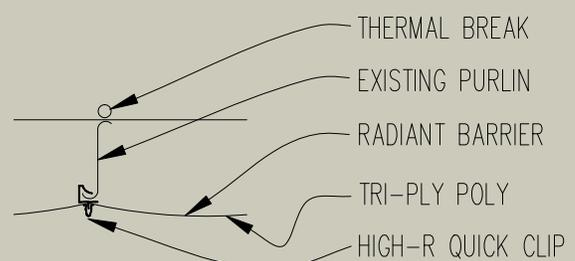
**HIGH-R® Poly Radiant Barrier Solution**
